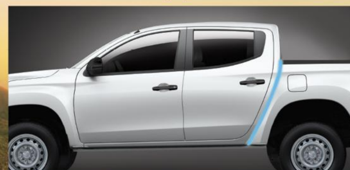
The J-line design is a clever engineering design made to shorten the wheelbase and maximize interior space.
