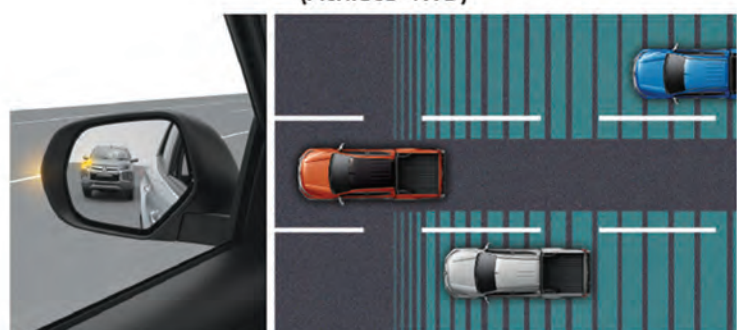
Blind Spot Warning System [BSW] with Lane Change Assist [LCA] (Athlete 4WD)
