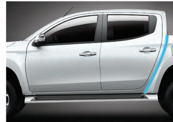
The J-line design is a clever engineering design made to shorten the wheelbase and maximize interior space
